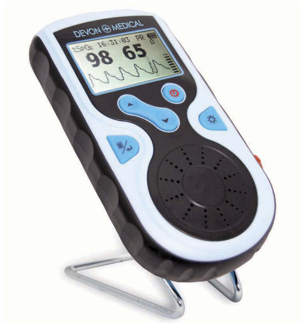
FIGURE 21.3 Portable pulse oximeter used to assess a pulmonary patient's arterial oxygenation. The number on the left of the display shows the percent saturation of hemoglobin in arterial blood ( S_aO_2 ), and the number on the right shows the HR.
